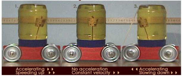
The tricky part is understanding image #3 in the picture above. When the accelerometer is moving in one direction and showing acceleration in the *opposite* direction, it is slowing down!
