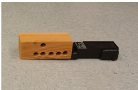
FIG. 2. Image from the block-push probe video, showing the battery-powered “car” (right) slowly pushing a wooden block at a constant speed to the left.
