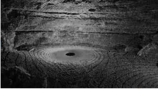
To better understand colony dynamics, researchers used a laser scanner to create a 3D representation of the bat cave.
